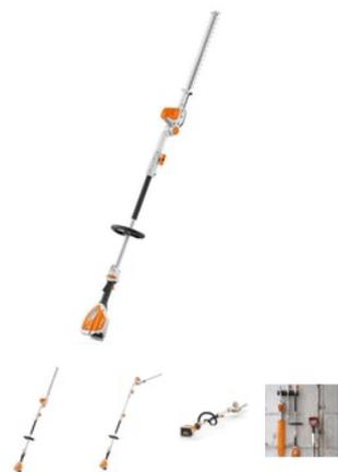
Lightweight 36V battery long-reach hedge trimmer for cutting taller hedges and shrubs in your home garden. Double-sided cutter blade in a droplet shape, variably adjusted blade angle from -45° to +90°, detachable shaft for easy transport. Carrying length: 115 cm. Total length: 210 cm.
