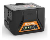
Lithium-ion battery for the STIHL AK-System with a voltage of 36V and a capacity of 180 Wh. Battery life depends on the device type. With charge level indicator (LED). Compatible with AL 101, AL 100, AL 300 and AL 500 chargers.
